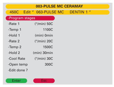
There are a total of six programmable stages. Five individually programmable heat rates, holding temperatures and holding times. The last stage is always designated as the cooling stage. The cooling stage is programmable and does feature an adjustable cool rate and open temperature.
