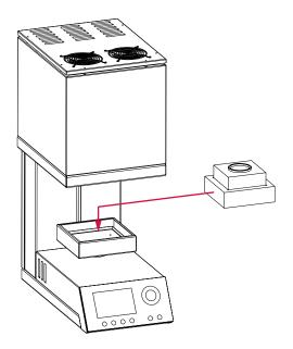
Once the lift is completely down, place the two insulation bases (see picture) on the lift plate.
