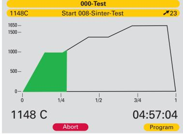
While the program is running, you can switch between parameter view and graph view by pressing the yellow button.
