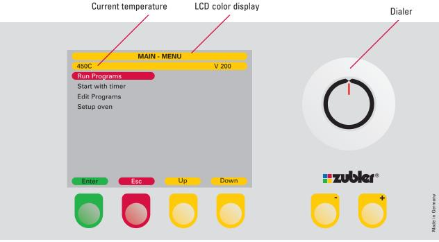
Section for selecting parameters: Confirm / Cancel - key Lift movement Up / Down
