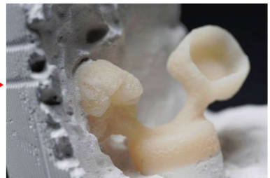
Figure 15: Result with strong reaction layer
