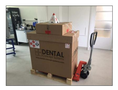
If possible unpack the machine at place where it shall be used. If this is not possible unpack the machine as described in chapter 3.1.3 "Unpacking" until the DC1 itself is left and carry the machine on the pallet to the final destination.
