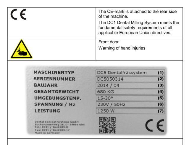
The type plate is attached to the rear side of the machine.
