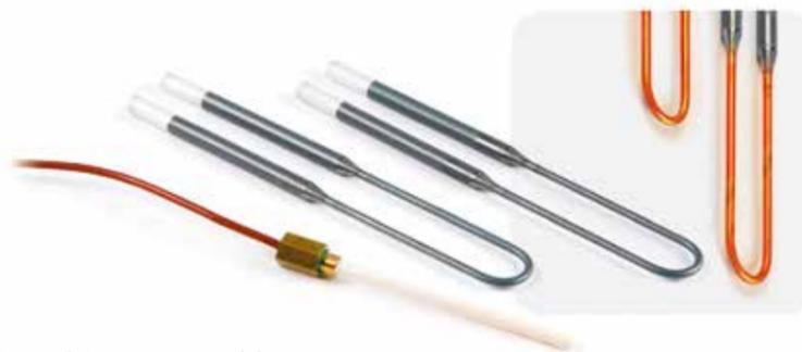
High-quality molybdenum disilicide heating elements reach a maximum end temperature of 1.650°C. Unlike silicon carbide heating systems, heaters of this type are far enough away from their maximum performance limit of approx. 1.800°C. Thanks to this property they attain a significantly longer service life. Each of the four heating elements can be individually replaced in case of damage – an „en bloc“ replacement is unnecessary.
