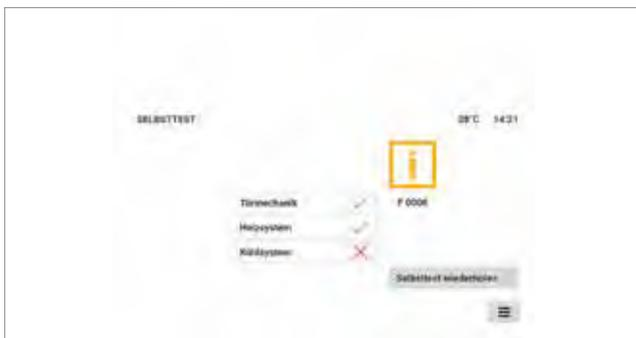
If there is an error, the corresponding error code is displayed. A red cross appears after the defective function. Follow the instructions on the screen.
