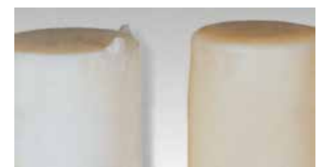
Typical marks of use and potential sources of error with Alox-plungers
