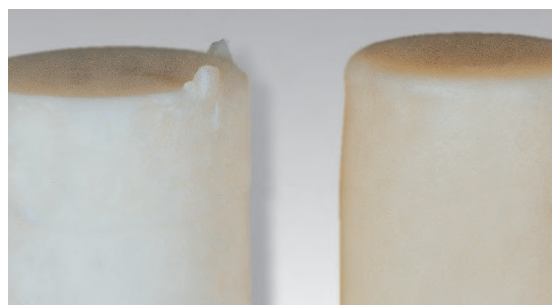
Typical signs of wear The source of problems with alumina oxide plungers
