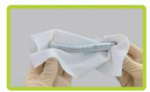
Step 5: After lubrication, run the dental handpiece to the normal speed to remove excess oil, and wipe off the residual oil on the surface.
