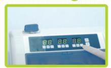
Step2:Select the cleaning mode of the high-speed /contra angle handpiece, and separately adjust and accurately control the filling time of each handpiece, which greatly reduces unnecessary waste of lubricating oil.
