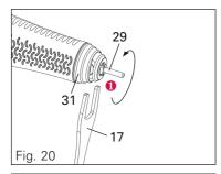
Clamp pin 29 or a milling bit. Turn the pin 29 until the flanks of the spindle 37 are visible at the tip 31 and the flat spanner 17 can be inserted.
