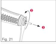
• Pull the tip 31 off the spindle 37 and insert the new spindle 37.
