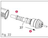
Make sure that the two spring holders **35** and the spring **36** are pushed onto the new spindle **37**. Make sure that the shoulder of each spring holder **35** is facing the spring **36**.
