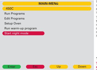
Instead of switching the furnace off, use night mode to prevent moisture and contamination from entering the firing chamber while the furnace is not in use.
