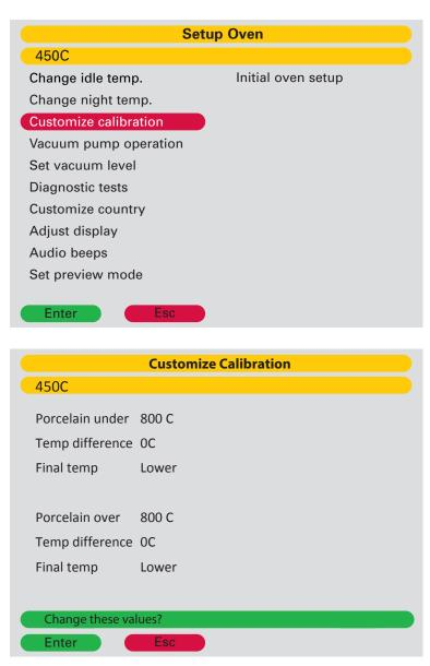
Users can offset their calibration for ceramic programs with final temperature above and/or below 800C all at once without adjusting programs individually effecting the actual calibration curve of the machine. This allows more precise offset modification of temperatures with the use of individually preferred temperature measurement methodology.
