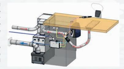
In practices or small laboratories with one or two technicians, dust can thus be extracted from the entire equipment space or work station area with one **Z2**. Use in alternative operation is particularly convenient. As long as only one suction station is in operation, the suction level can be selected as with a single-station suction system and can be individually saved for each work station.
