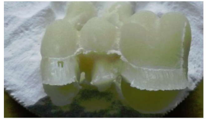
Figure 2: improper milling wax was used
