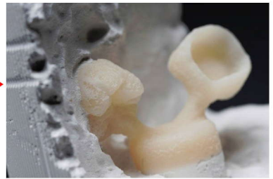
Figure 15: Result with strong reaction layer
